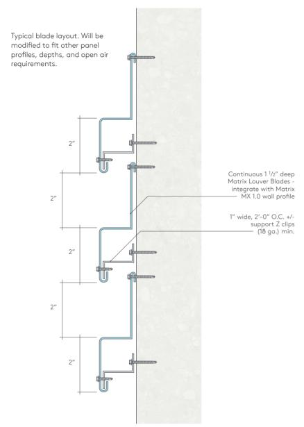
Morin fabricates cosmetic or nonfunctioning louver options matching virtually all panel series available. Louvers can be designed to allow a predetermined open area for specific projects ventilation requirements.
